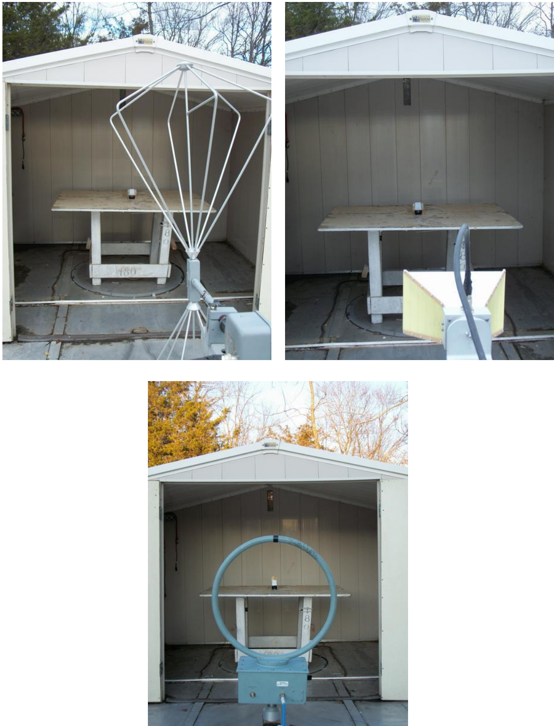
Figure 3.1 Radiated Test Setup
