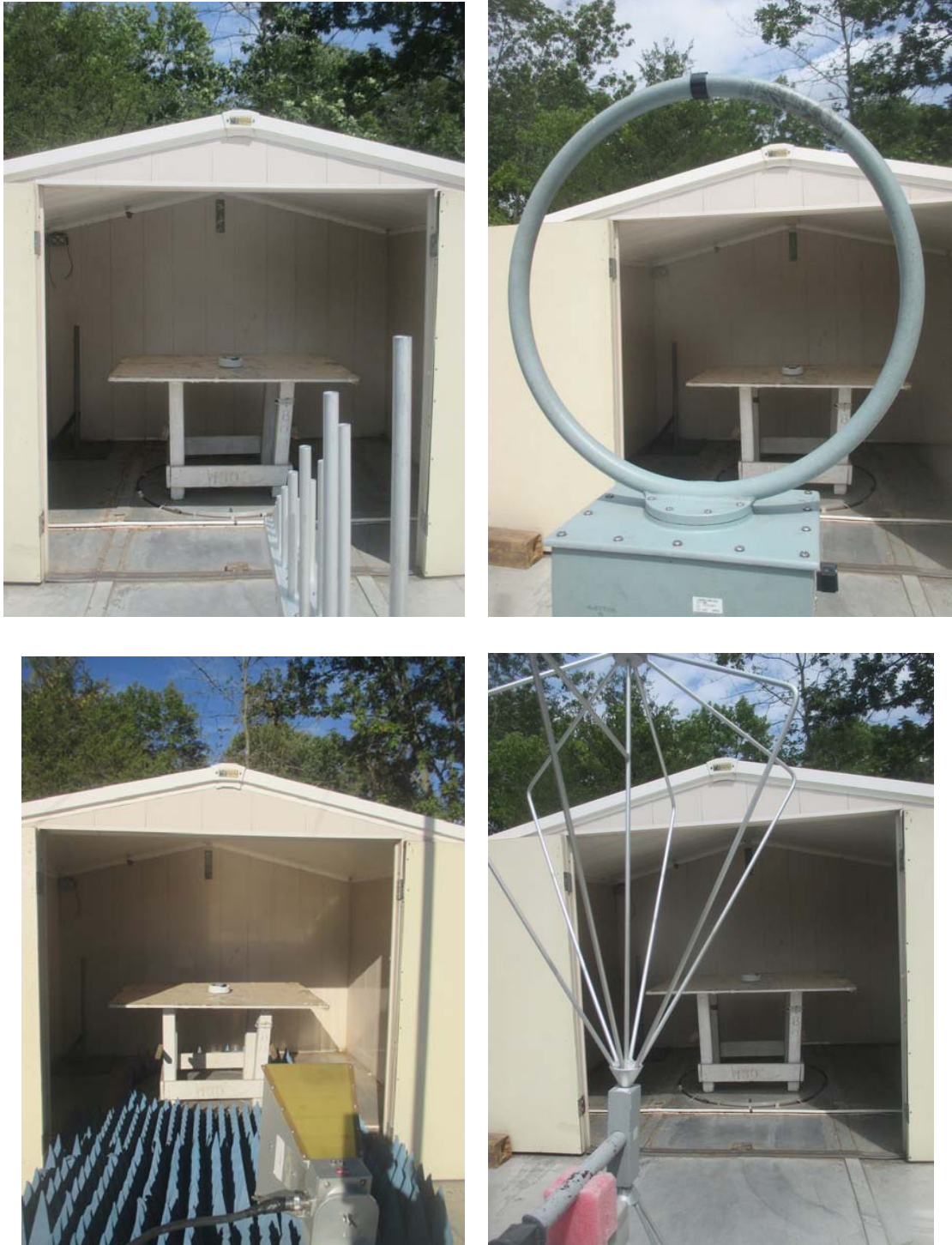
Figure 3.1 Radiated Test Setup
