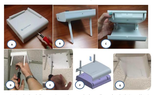
Attach a Star Ceiling mounting attachment to the drop-ceiling track at the designated location.
