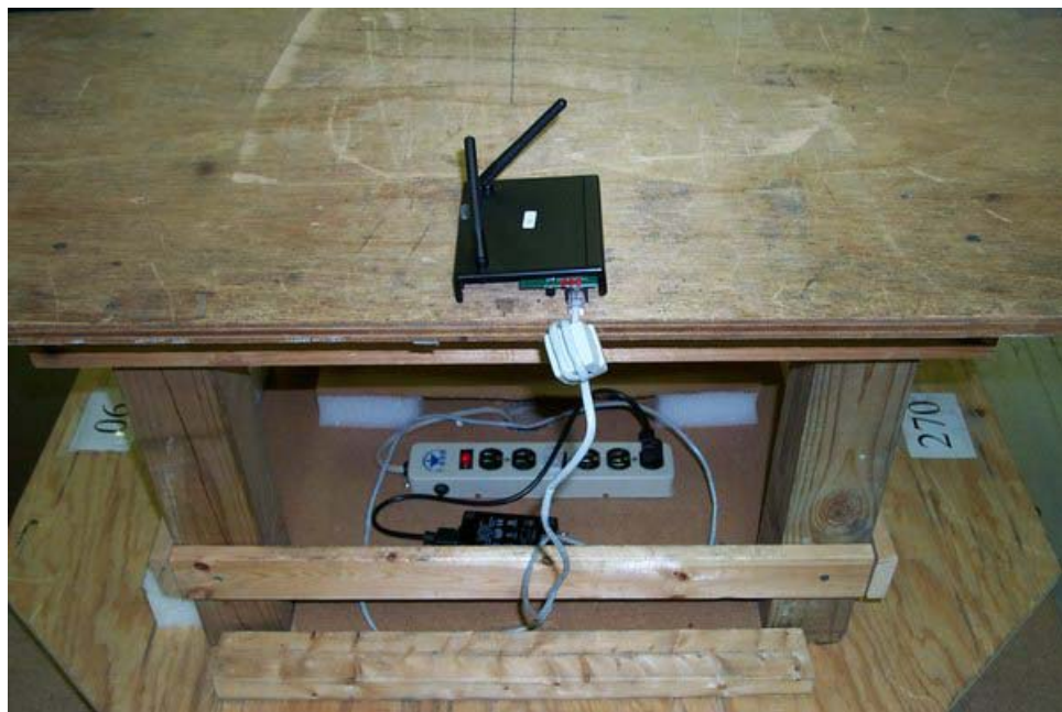
Figure 3.1 Radiated Test Setup ( Power option: AC/DC Adaptor or Power Ethernet)
