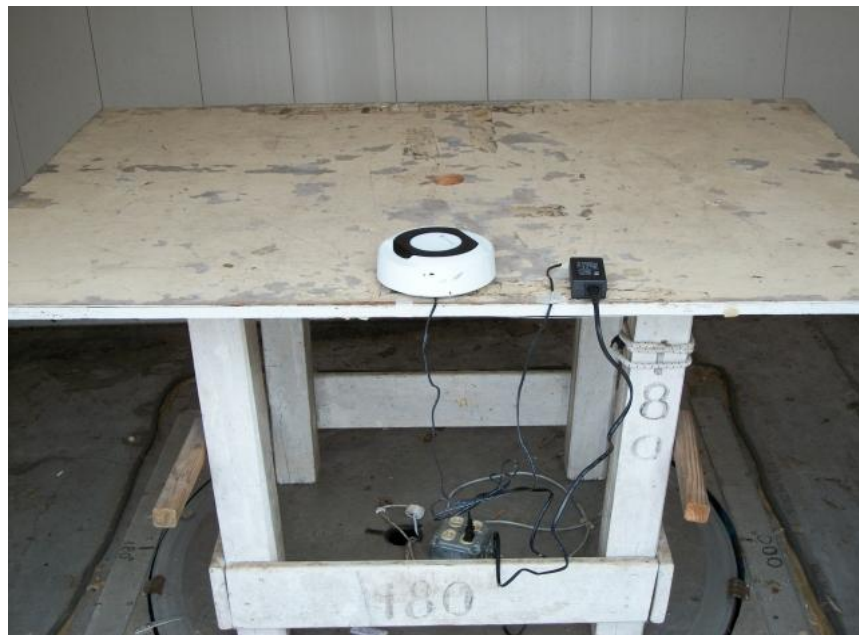
Figure 3.2 Radiated Test Setup, AC Mode
