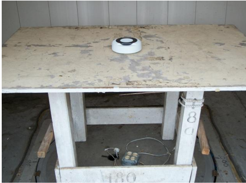
Figure 3.1 Radiated Test Setup, Battery Mode
