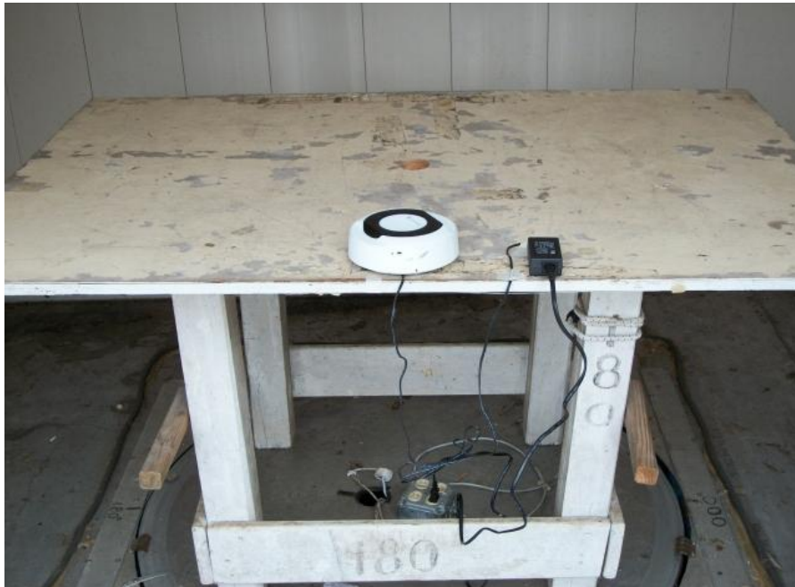
Figure 3.2 Radiated Test Setup, AC Mode
