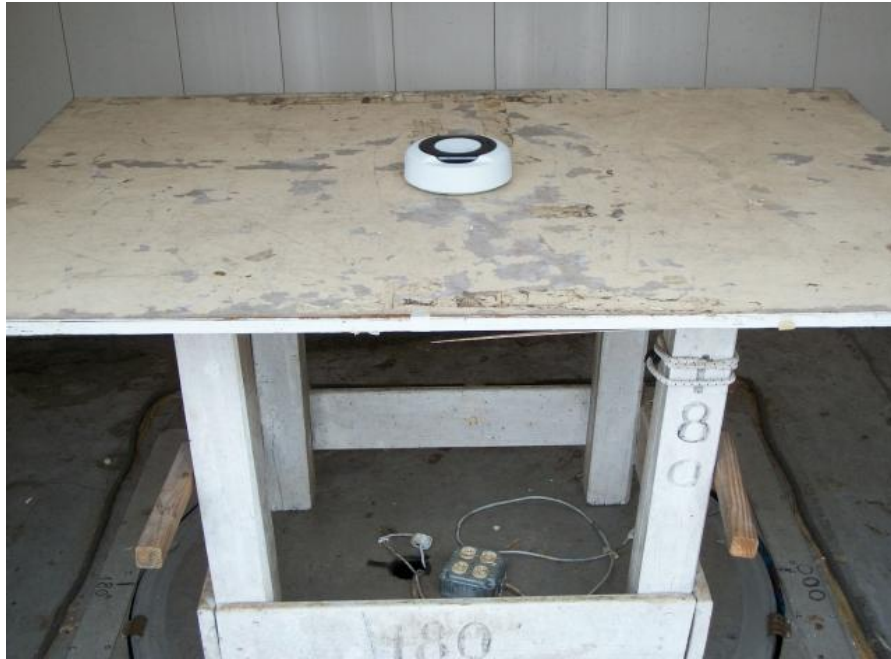
Figure 3.1 Radiated Test Setup, Battery Mode
