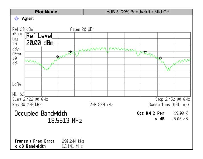
EUT: 2.4GHz DTS Transmitter Module Report No: 0048-130114-03 Model: CEN-8B FCC ID:ST2-CEN8B IC: 6012A-CEN8B
