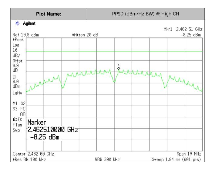
EUT: 2.4GHz DTS Transmitter Module Report No: 0048-130114-03 FCC ID:ST2-CEN8B IC: 6012A-CEN8B Model: CEN-8B
