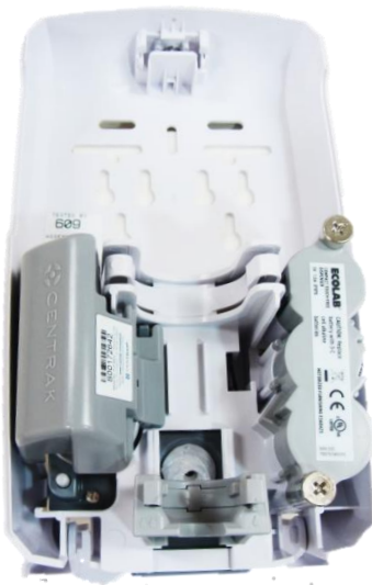
IT-373ECO shown integrated with a Ecolab Dispenser
