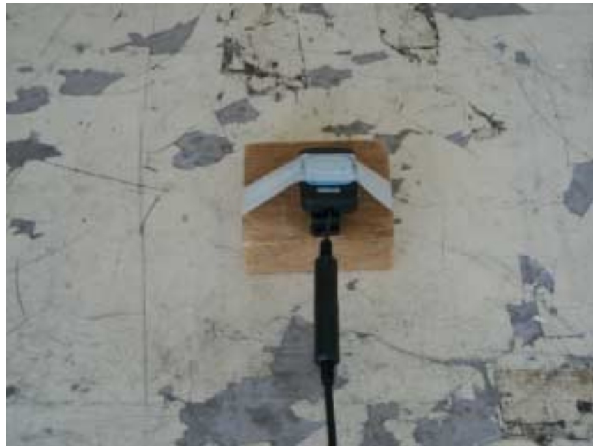
Figure 3.1 Radiated Test Setup, position 1
