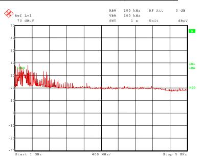
The following additional frequencies were found during the preliminary radiated emission test: 1299.1575 MHz and 1732.21 MHz.
