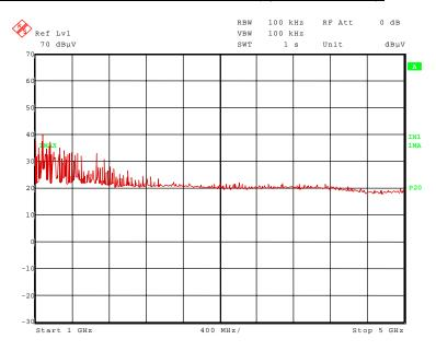
The following frequencies were found during the oven measurement (transmitter not installed): 1.020 GHz, 1.060 GHz, 1.100 GHz, 1.140 GHz, 1.333 GHz and 1.416 GHz.
