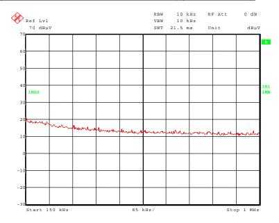
No significant additional frequencies above the noise floor of the system and the measurement results without transmitter were found during the preliminary radiated emission test, so no measurements were carried out on the outdoor test site.
