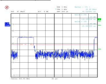
Length of period = 177.88  $\mu$ s, length of pulse = 41.644  $\mu$ s, number of transmissions = 492 (87.452 ms / 177.88  $\mu$ s).
