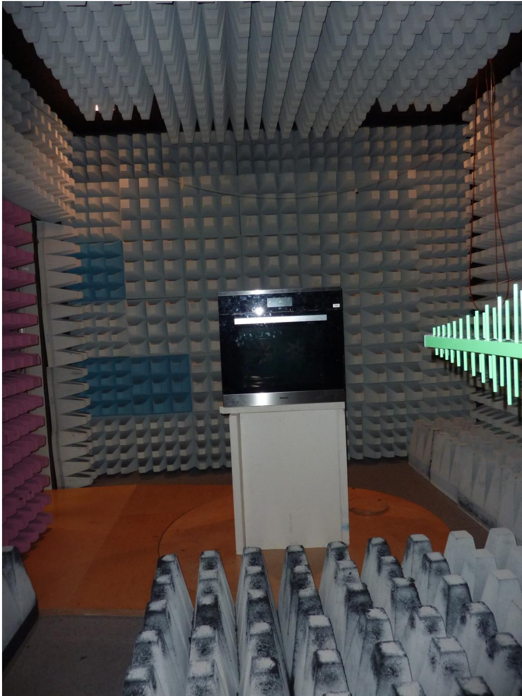
132604_2_1.JPG: EPI7674 inside H6880BP, test set-up fully anechoic chamber
