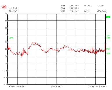
132604\_36.wmf: Spurious emissions from 30 MHz to 230 MHz (operation mode 1):
