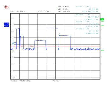
The complete pulse train consists of 6 (3 for resonator 1 and 3 for resonator 2) sub pulse trains with different transmit power. The time for transmitting for the different resonators is always the same.
