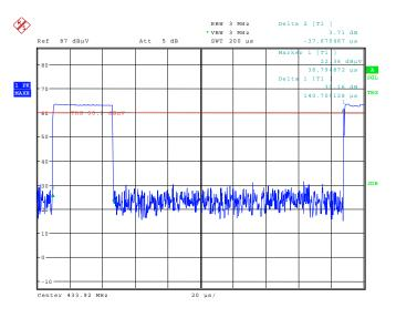
Length of period = 178.34  $\mu$ s, length of pulse = 36.795  $\mu$ s, number of transmissions = 526 (93.891 ms / 178.34  $\mu$ s).
