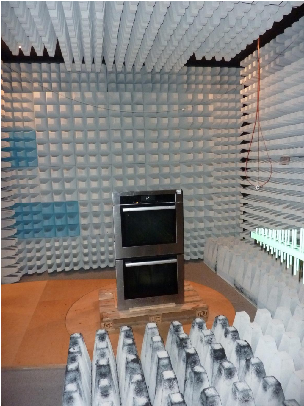
132604_3_4.JPG: EPI7674 inside H6780BP2, test set-up fully anechoic chamber
