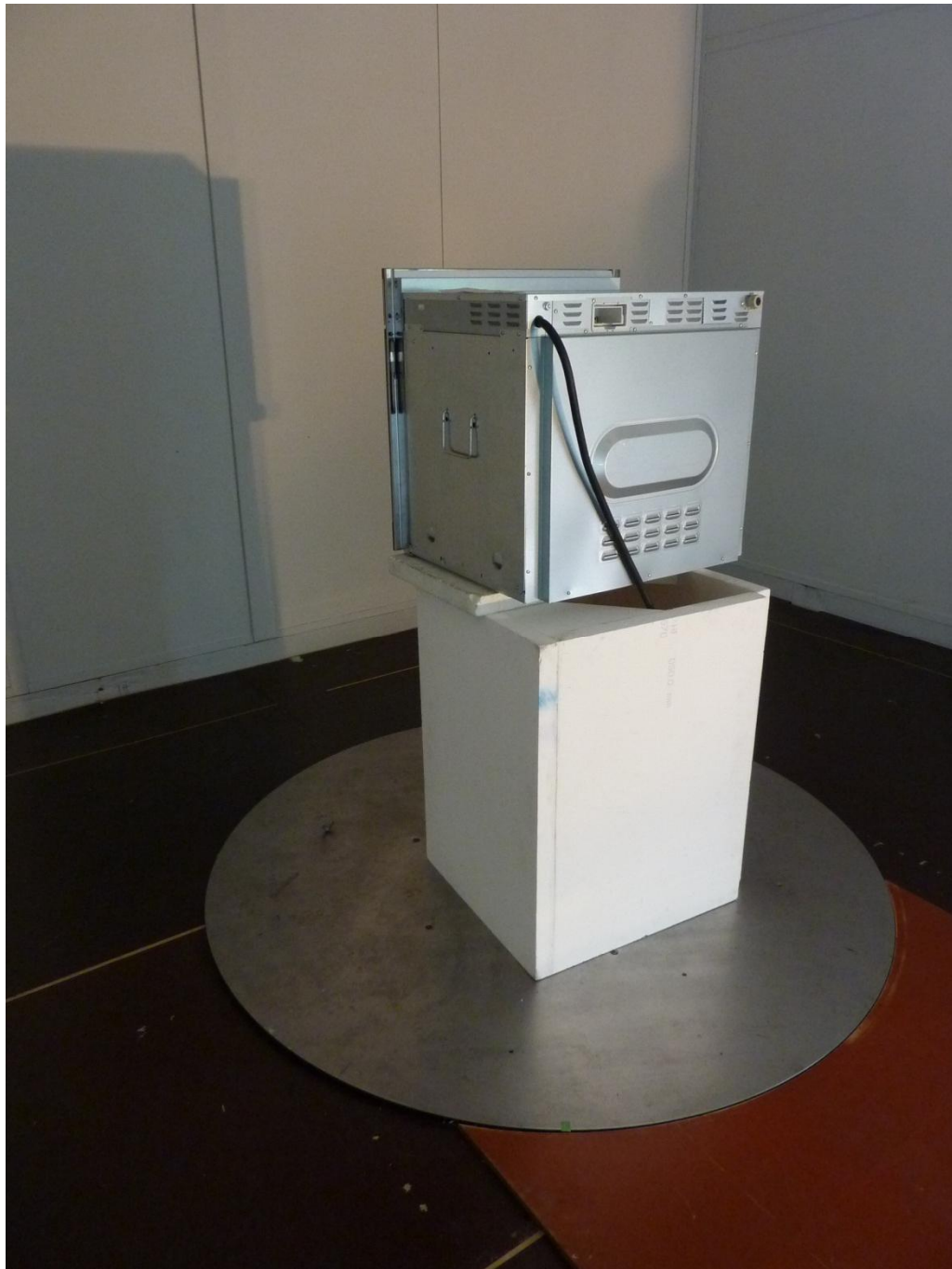
132604_1_3.JPG: EPI7674 inside H6780BP, test set-up open area test site
