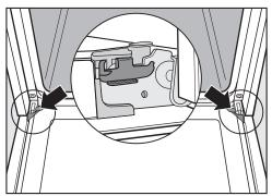
The door is connected with brackets on each door hinge.
