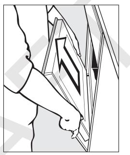
Holding the door securely at both sides, lift it straight upwards.
