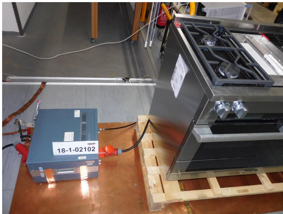
Photograph 4: Conducted emission on the AC port Set Up
