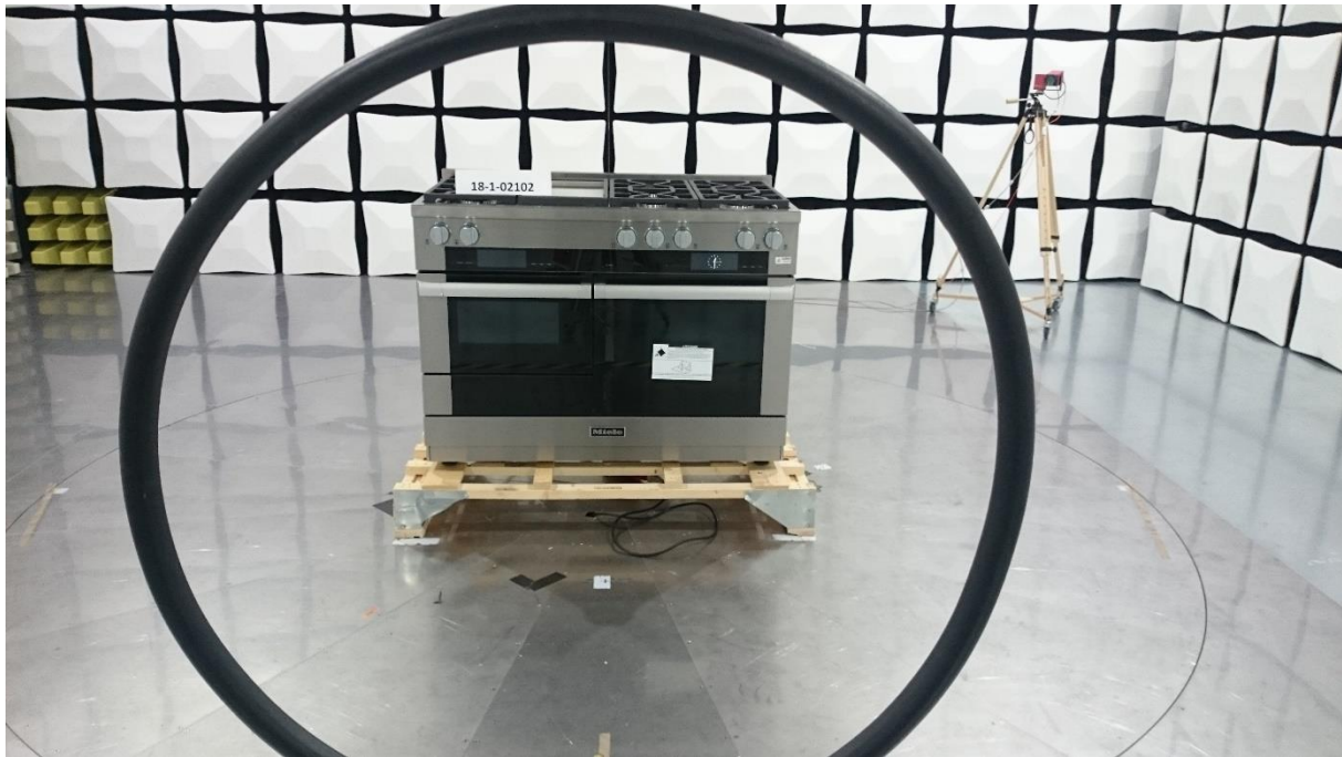
Photograph 5: Set Up - Front side Overall View- 9 kHz-30 MHz- Front Side
