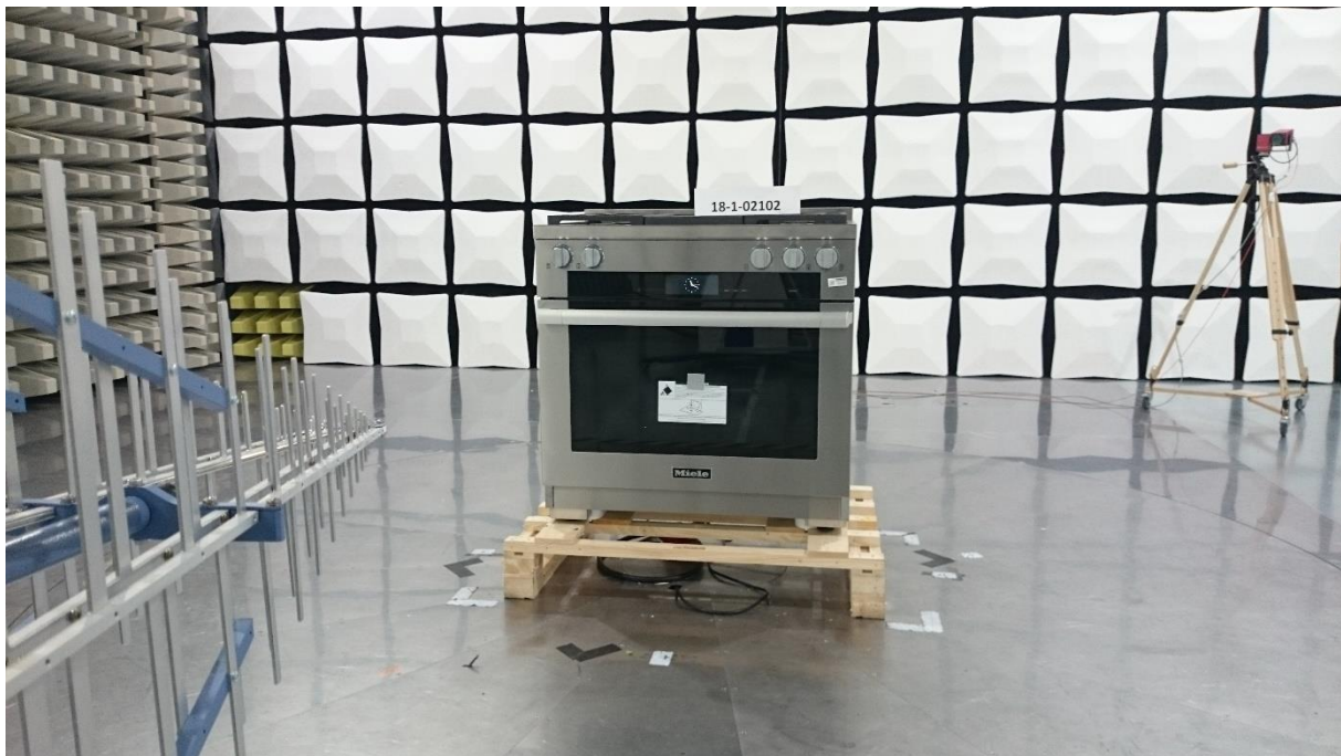
Photograph 6: Set Up -overall View- above 30MHz - EUT 0° - Front Side
