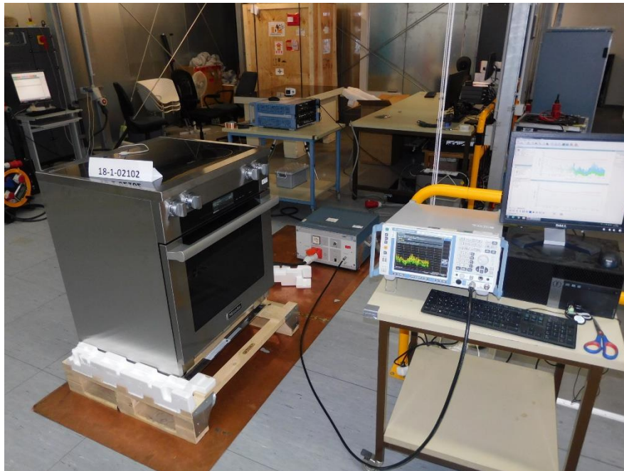
Photograph 3: Conducted emission on the AC port Set Up
