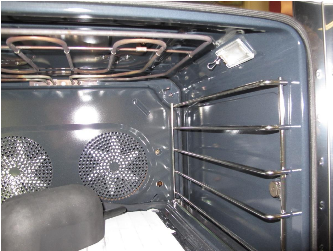
Photograph 8: Loop Antenna placement in the cavity
