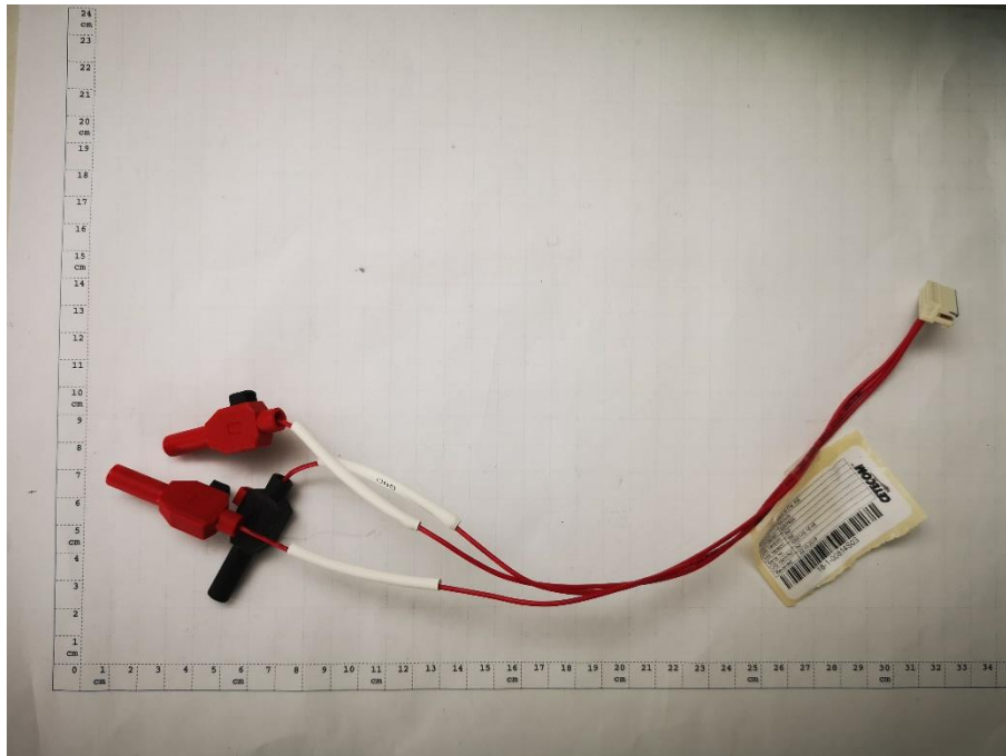
Photograph 11: AE 1 - DC power Cable for Module Adapter
