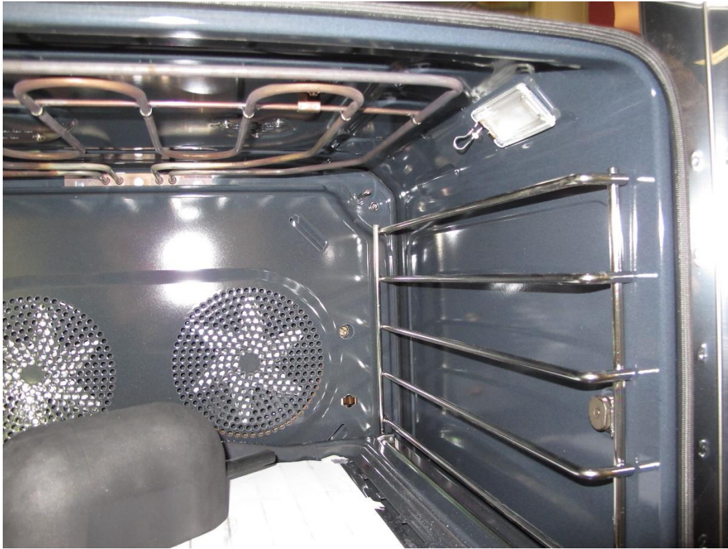
Photograph 9: Loop Antenna placement in the cavity
