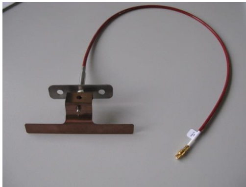
Picture 3: rod antenna with the coupling plate, mcx-connector
