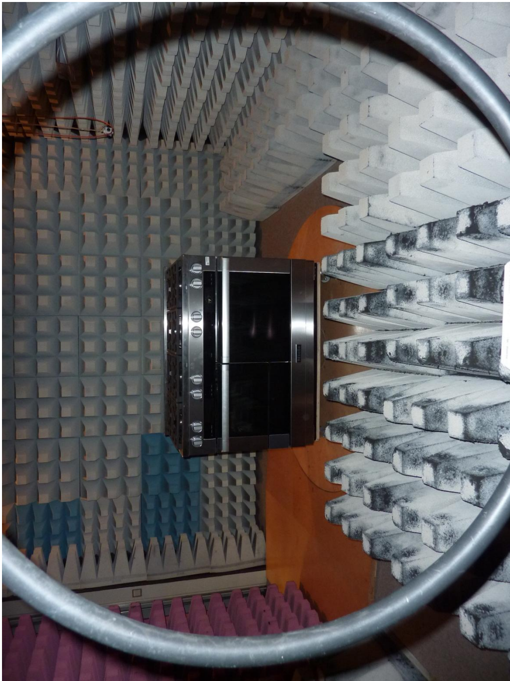
136015_3_5.JPG: EPI7674 inside HR1954, test set-up fully anechoic chamber
