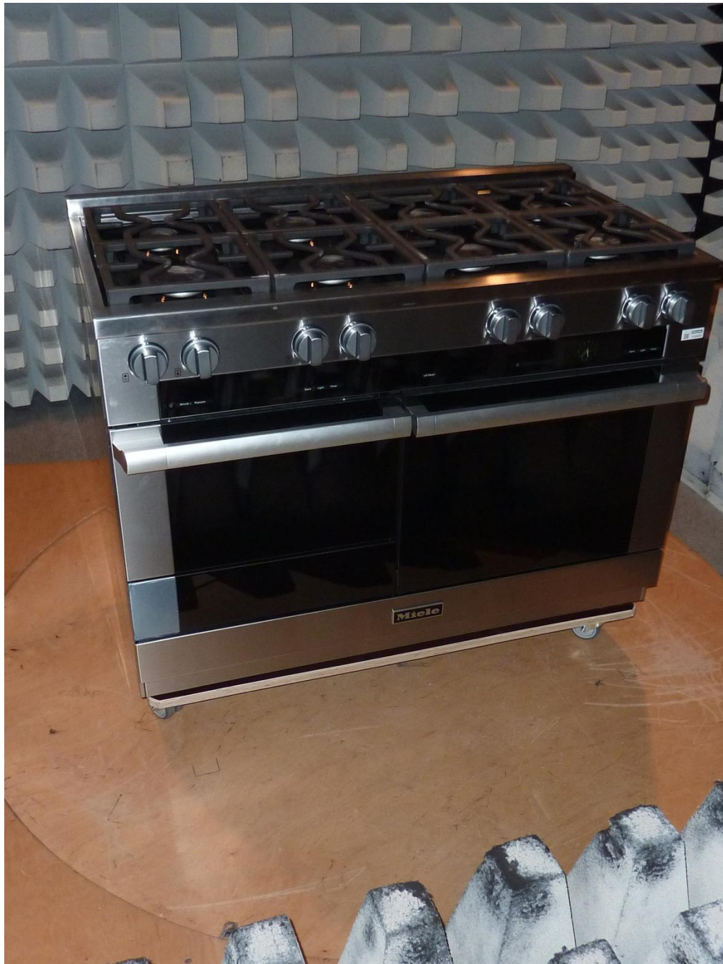
136015_3_2.JPG: EPI7674 inside HR1954, test set-up fully anechoic chamber
