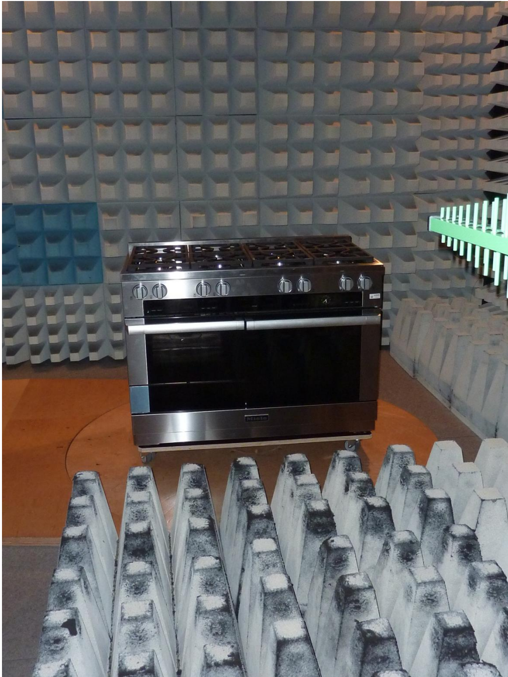
136015_3_1.JPG: EPI7674 inside HR1954, test set-up fully anechoic chamber
