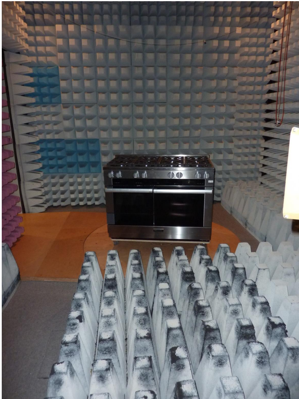
136015_3_4.JPG: EPI7674 inside HR1954, test set-up fully anechoic chamber
