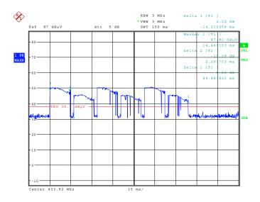
The complete pulse train consists of 6 identical sub pulse trains which may differ in transmit power (belongs on the used food probe).
