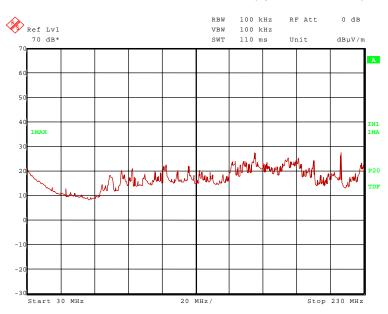
136015\_34.wmf: Spurious emissions from 30 MHz to 230 MHz (operation mode 2):
