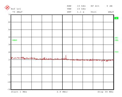
The following frequency was found during the oven measurement (transmitter not installed): 16.517 MHz.
