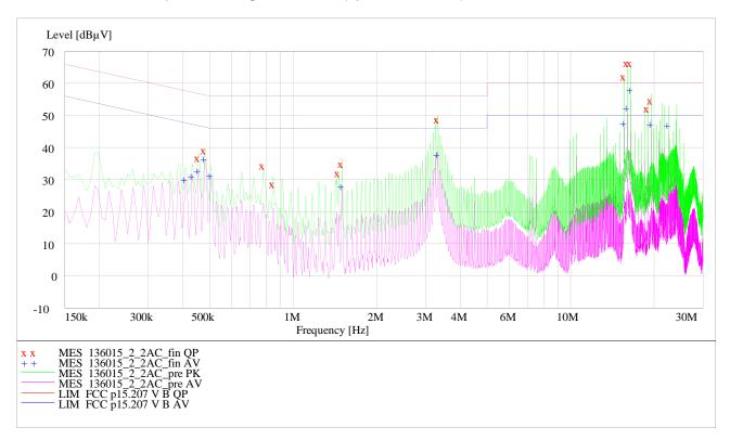
136015\_2\_2AC: EUT operates on highest channel (operation mode 2):
