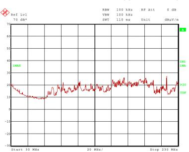
136015\_32.wmf: Spurious emissions from 30 MHz to 230 MHz (operation mode 1):
