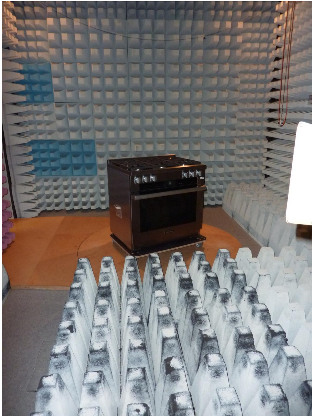
136015_2_5.JPG: EPI7674 inside HR1934, test set-up fully anechoic chamber
