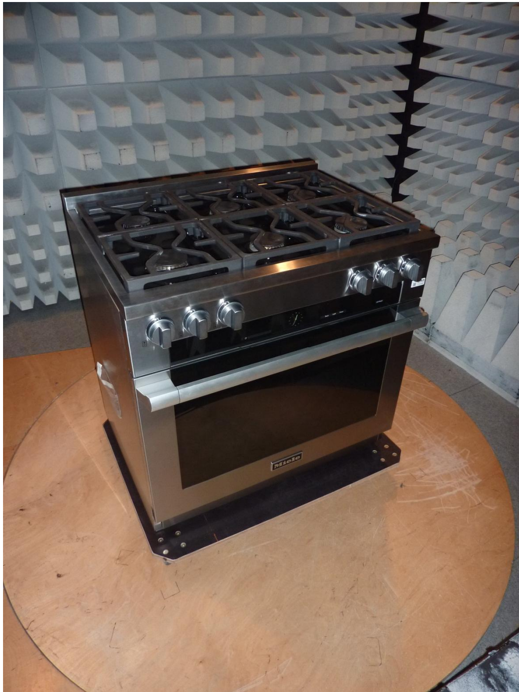
136015_2_3.JPG: EPI7674 inside HR1934, test set-up fully anechoic chamber
