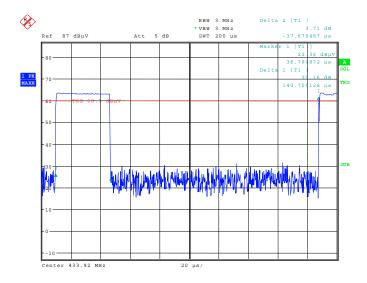
Length of period = 178.34  $\mu s,$  length of pulse = 36.795  $\mu s,$  number of transmissions = 526 (93.891 ms / 178.34  $\mu s).$
