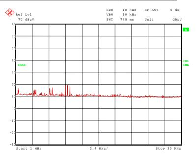
The following frequencies were found during the oven measurement (transmitter not installed): 1.495 MHz, 4.485 MHz, 7.475 MHz and 10.044 MHz.
