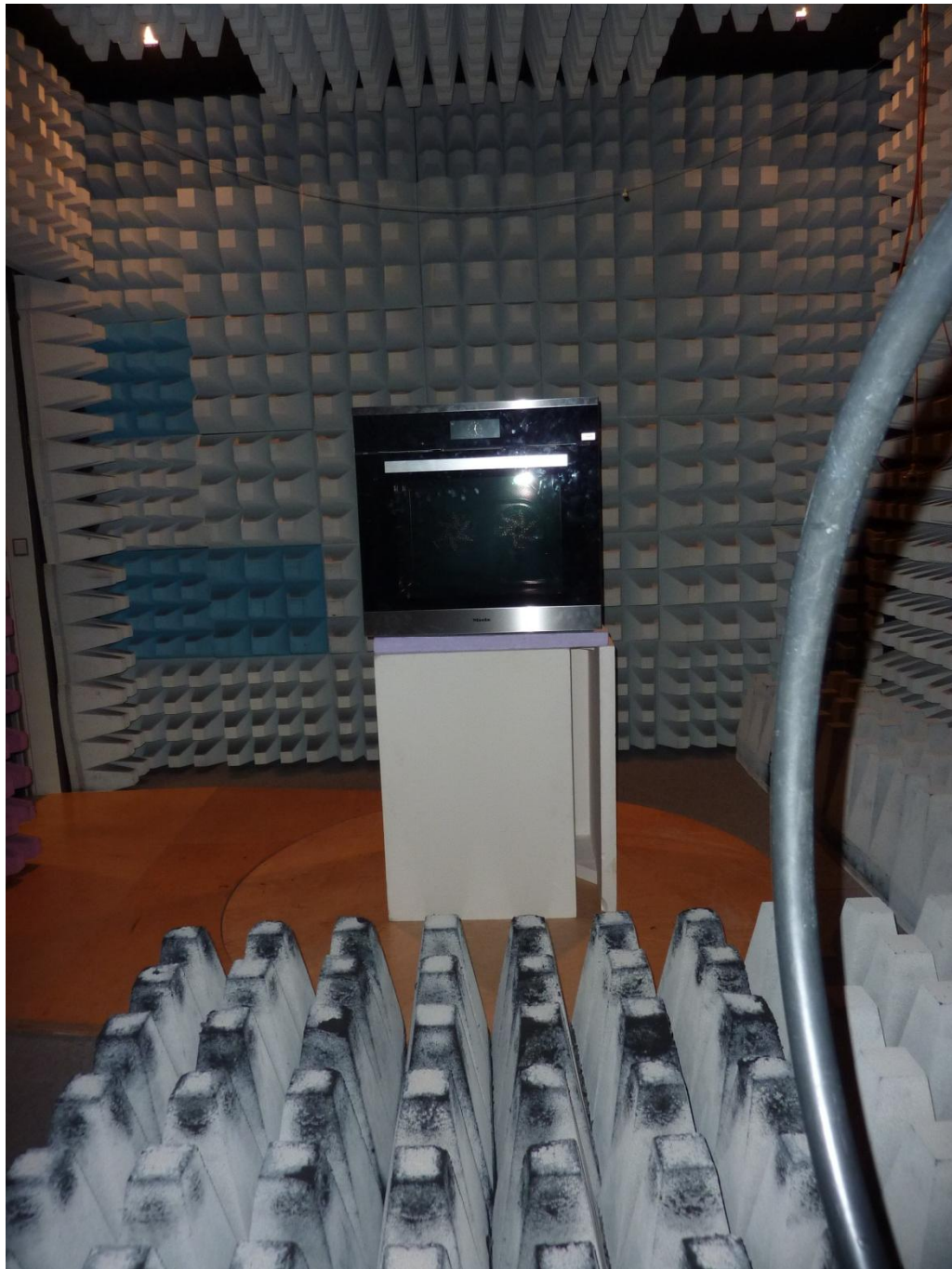
132604_2_7.JPG: EPI7674 inside H6880BP, test set-up fully anechoic chamber
