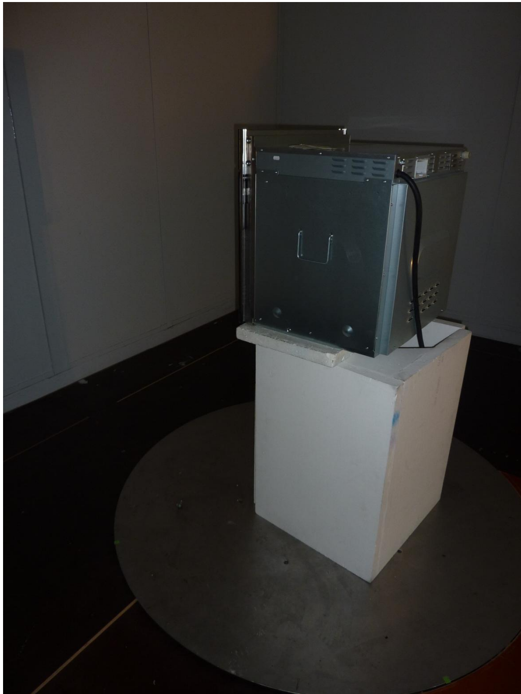
132604_2_3.JPG: EPI7674 inside H6880BP, test set-up open area test site
