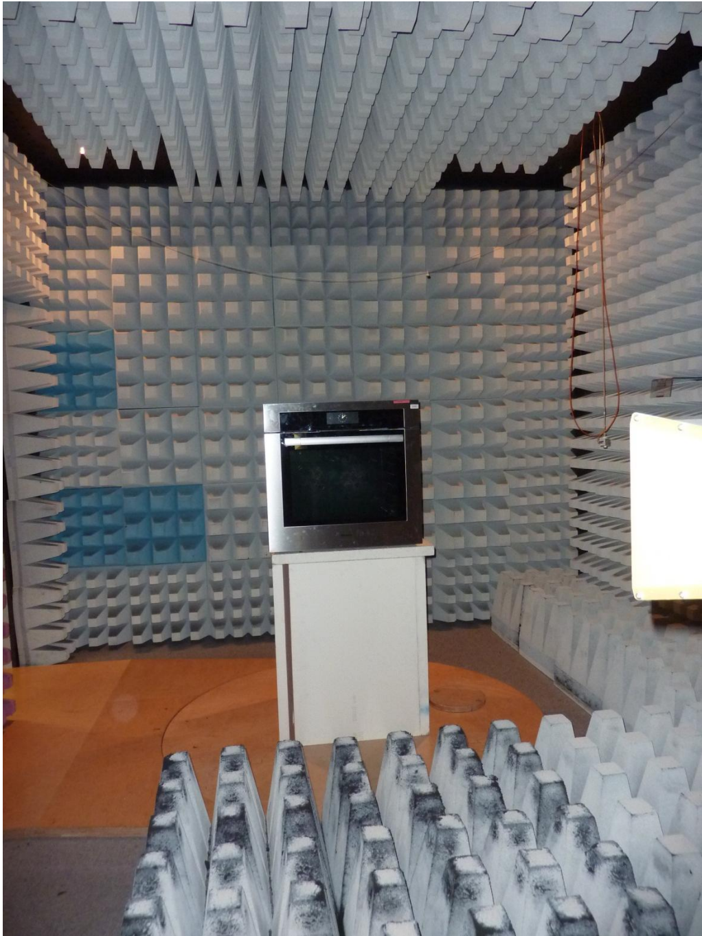
132604_1_2.JPG: EPI7674 inside H6780BP, test set-up fully anechoic chamber
