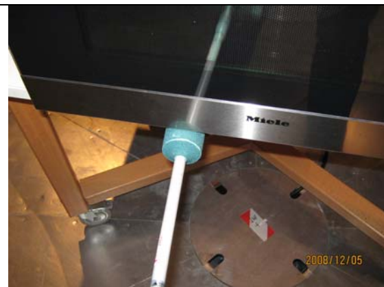
Fig. 1b Radiation leakage test after door adjustment
