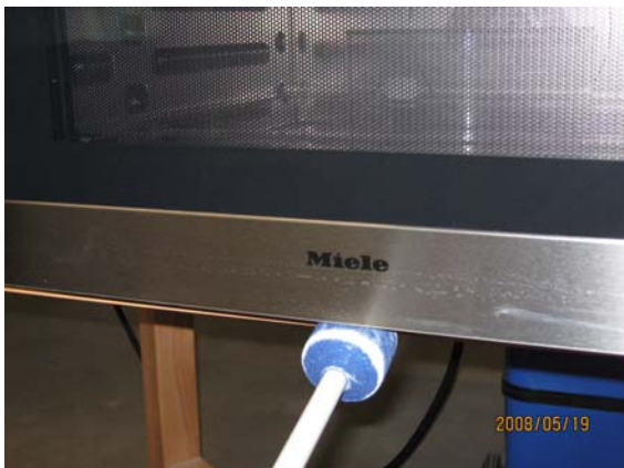
Fig. 1 Radiation leakage test
