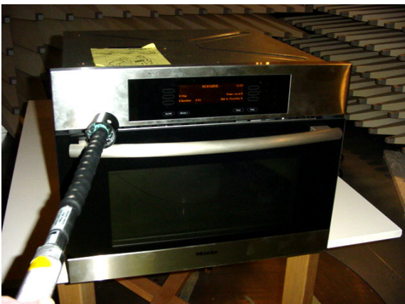
Fig. 1 Radiation leakage test
