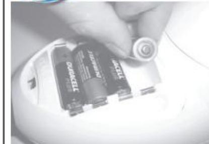
Fit only new batteries taking great care to ensure the correct polarity and the contacts are clean and made correctly as some batteries may differ in size and form
