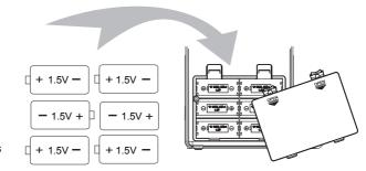
Battery: USE SIX SIZE "C" or UM-2 1.5V BATTERIES
