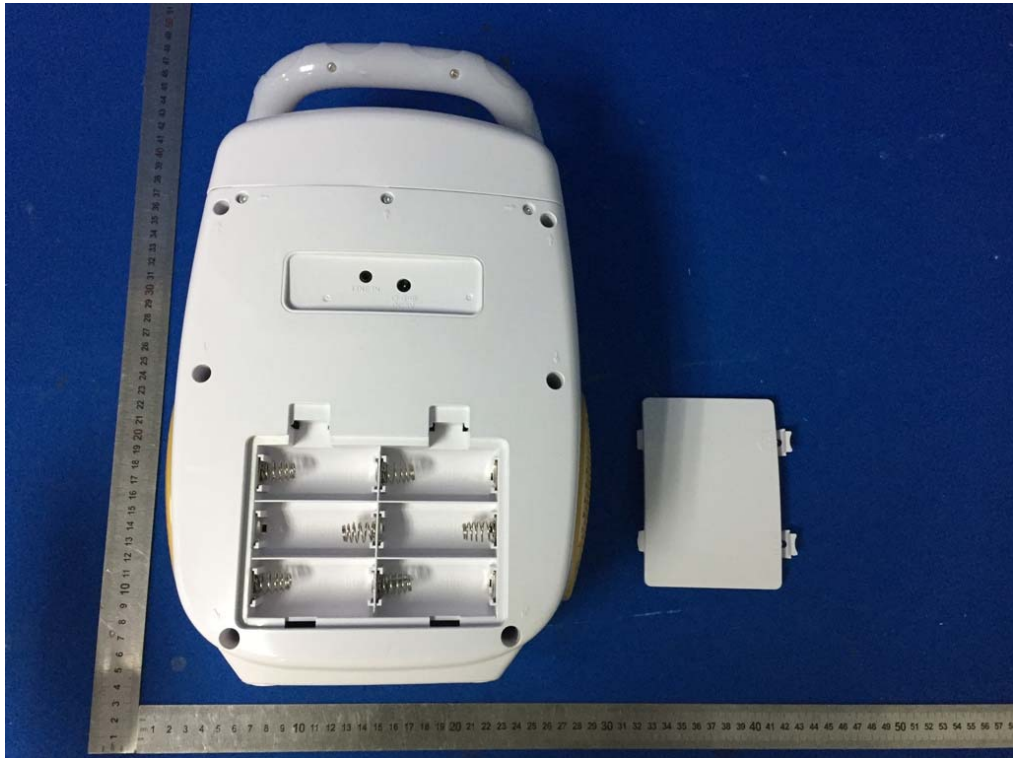
Fig. 9 Battery view of main unit
