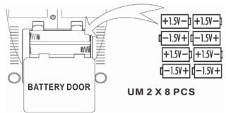
Fit 8 x 1 .5V C-size batteries (not included), referring to the polarity markings inside the battery compartment. Never mix old and new batteries. Finally, replace the cover.
