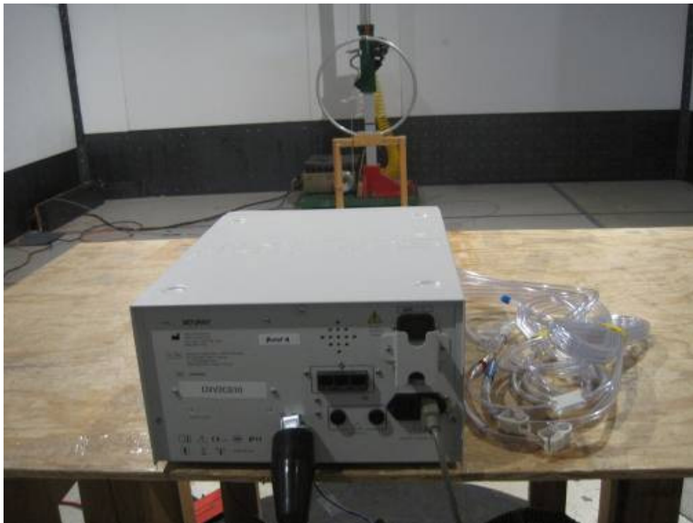
Radiated Emission<30MHz Test Setup – Rear View
