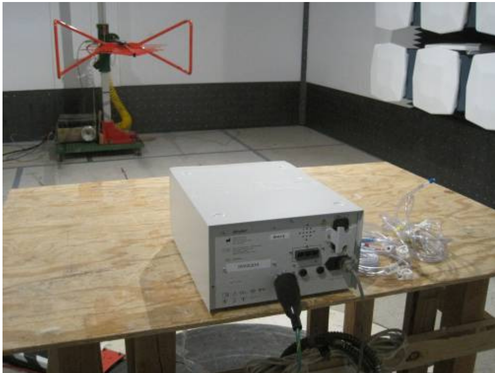
Radiated Emission>30MHz Test Setup – Rear View
