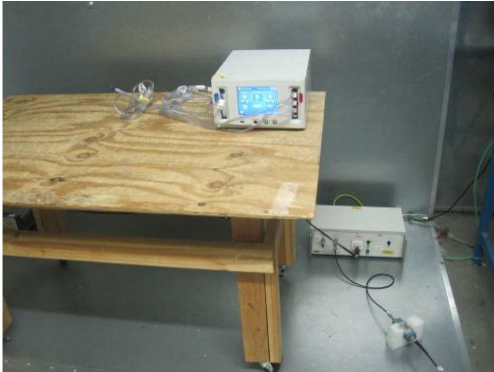
Conducted Emission Test Setup – Front View
