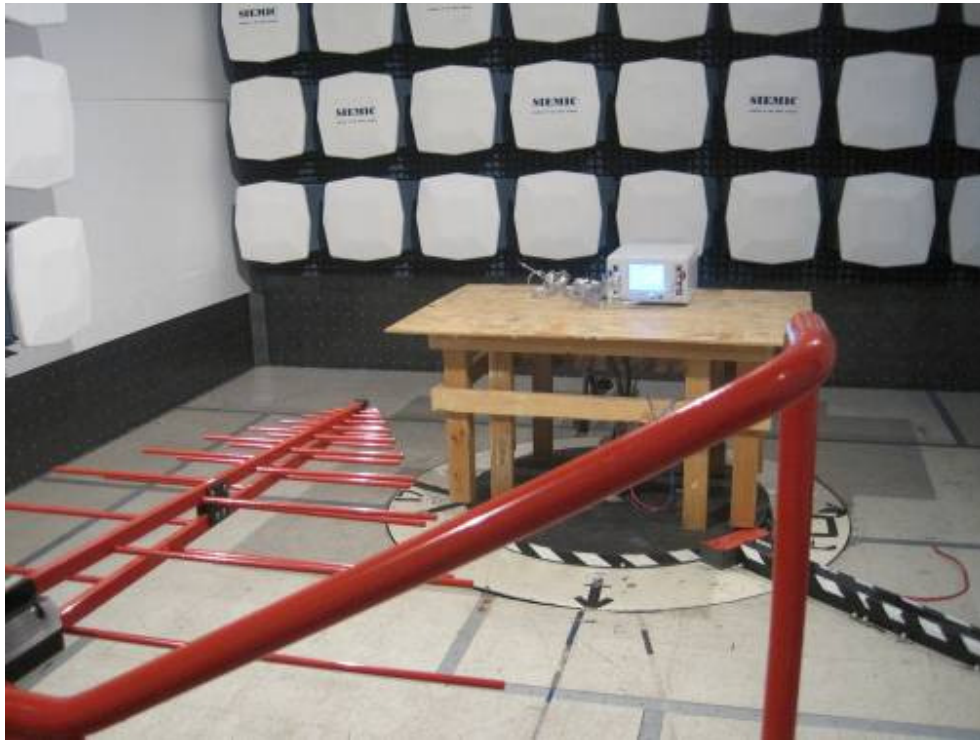
Radiated Emission>30MHz Test Setup – Front View
