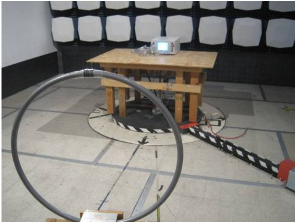
Radiated Emission<30MHz Test Setup – Front View
