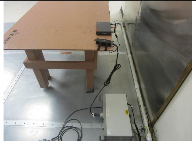
Conducted Emission Test setup – Rear View
