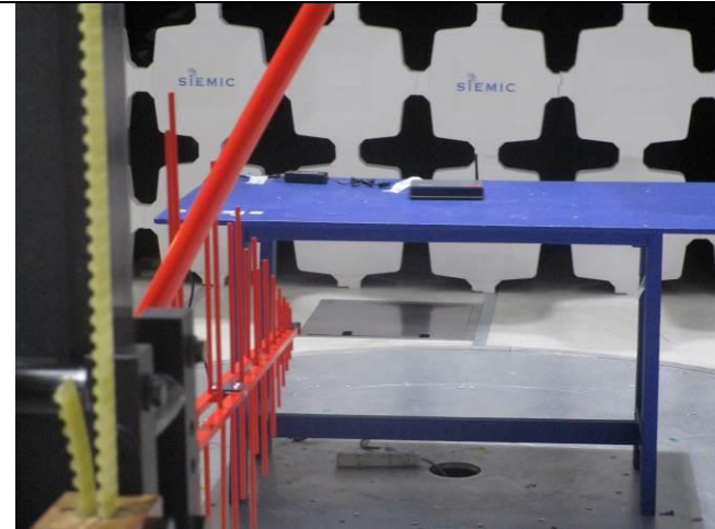
Radiated Emission Test setup (<1GHz) – Front View
