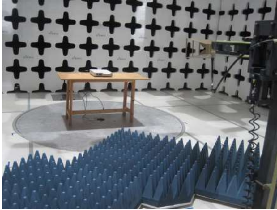
Radiated emissions above than 1 GHz setup - Front view
