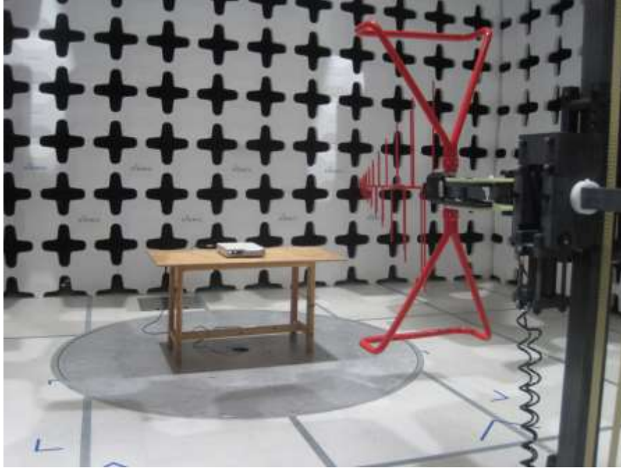
Radiated emissions below 1 GHz setup - Front view
