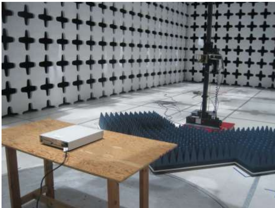
Radiated emissions above than 1 GHz setup - Back view
