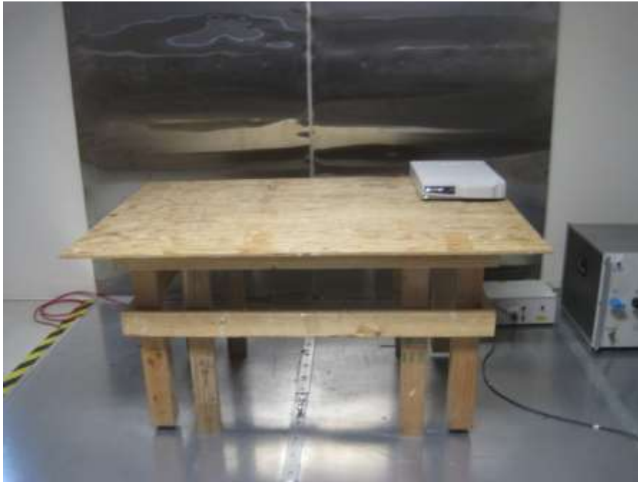
Conducted emissions Test Setup - Front view
