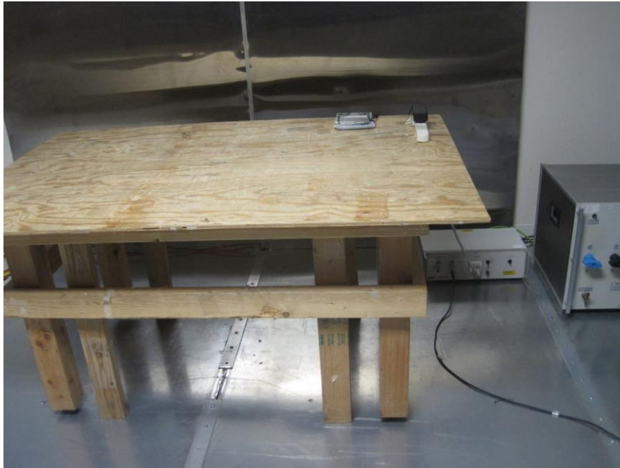
Conducted emissions Test Setup - Front view
