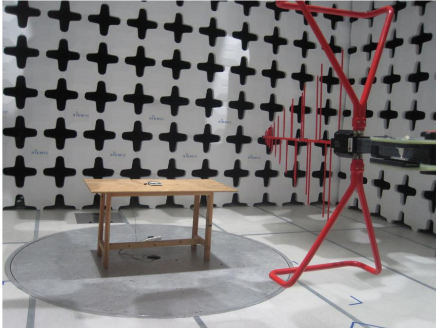
Radiated emissions below 1 GHz setup (Receiver module) - Front view
