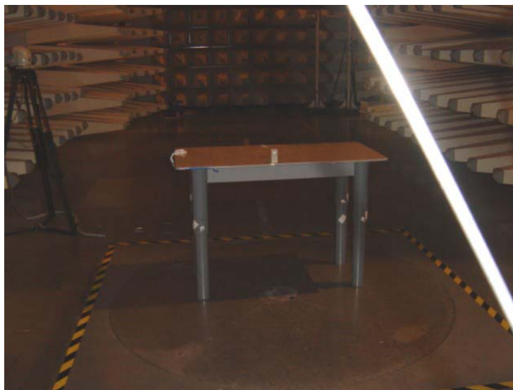
Set-up for Radiation Emission ( Transmitter)
