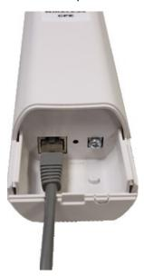
3. Slide the cover back and press down the lock button to seal the bottom of the JetWave 2450v2.
