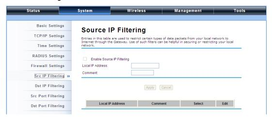
You may create and activate a rule that filters a packet based on the source IP address from your local network to Internet. Check "Enable Source IP Filtering" to activate rule.
