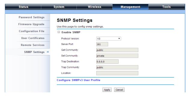
**Protocol Version**: Select the SNMP version, and keep it identical on the IEEE 802.11n JetWave 2450v2 and the SNMP manager. The IEEE 802.11n JetWave 2450v2 supports SNMP v2/v3.
