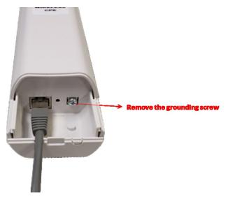
2. Put the grounding wire on the grounding point at the bottom of the JetWave 2450v2. Then screw the grounding wire to tighten up.
