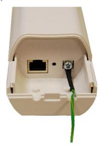
3. Connect the grounding wire to earth ground.
