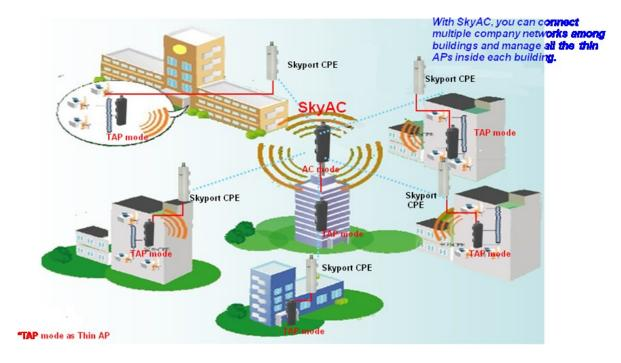
When a thin AP mode joins a wired network, it will start to look for a JetWave 2450v2 in AC mode. If the thin AP founds the AP controller on the network, it will send the registration request to the AP controller. Once the registration is successfully made, the AP that acts as the AP controller will add the thin AP to its management list and provides it configuration information.
