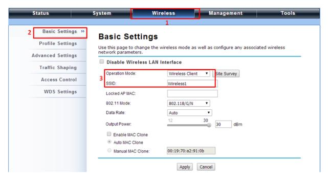
Besides specifying the SSID manually, you may select the preferable Access Point to connect by clicking the "Site Survey" button beside Wireless Mode. Once the button is pressed, the wireless client will scan all the available access points within coverage. Select the one you prefer to connect, and click Select AP to establish the connection.
