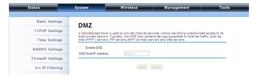
**DMZ Host IP Address:** Enter the local host IP address.
