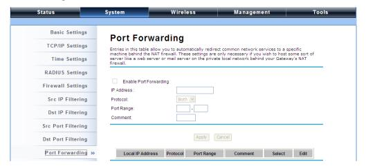
The port forwarding allows you to automatically redirect common network services to a specific machine behind the NAT firewall. These settings ne are only necessary if you wish to host some sort of server like a web server or mail server on the private local network behind IEEE 802.11n Wireless JetWave 2450v2's NAT firewall. Check the **Enable Port Forwarding** checkbox to
