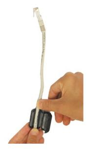
3. Loop the cable around and through the core. This helps "lock" the core in place, and may be required in circumstances with severe interference.
