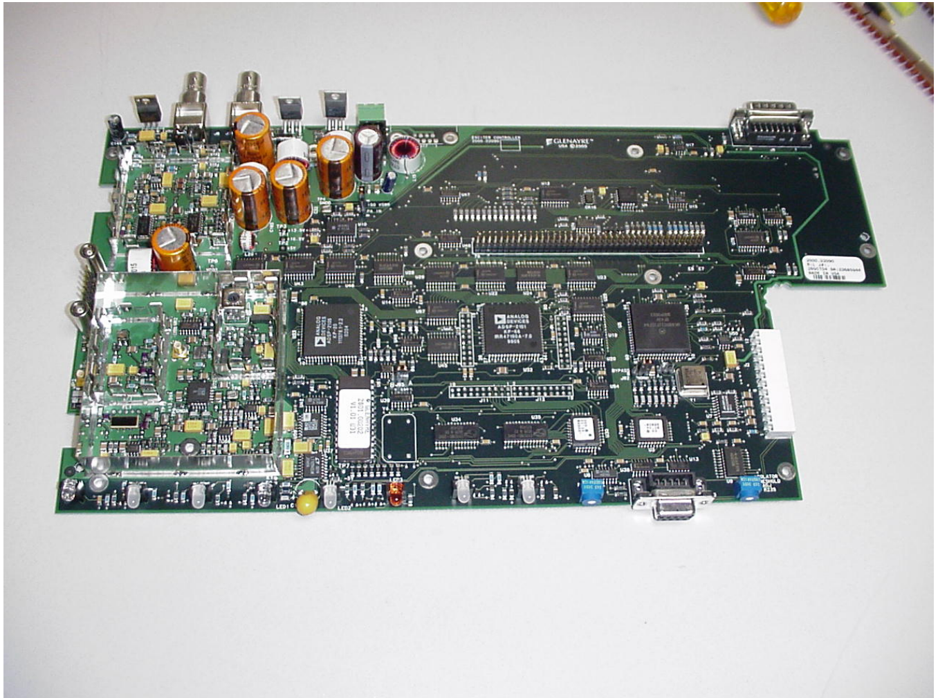
2000.02090 DSP Exciter Control Board (covers removed)
