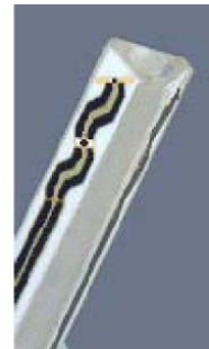
Figure E.2.2 Probe Thick-Film Technique
