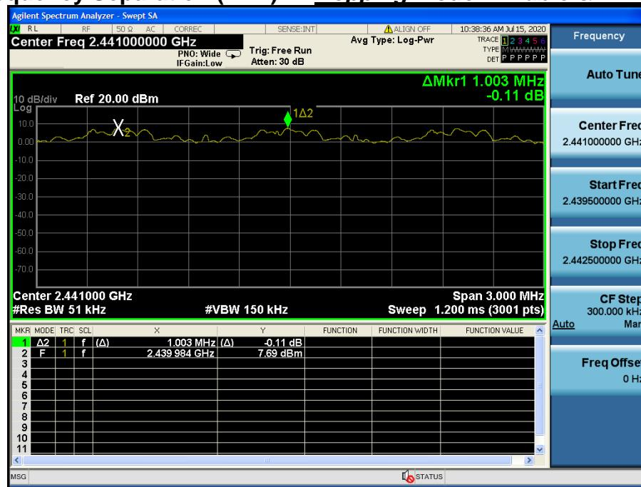
**Carrier Frequency Separation (AFH)      Hopping mode : Enable & 8DPSK**
