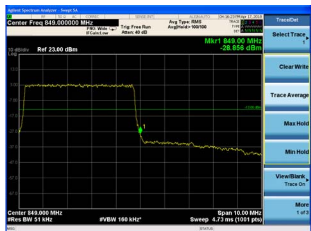
LTE Band 5 16QAM 5MHz CH-High 100%RB
