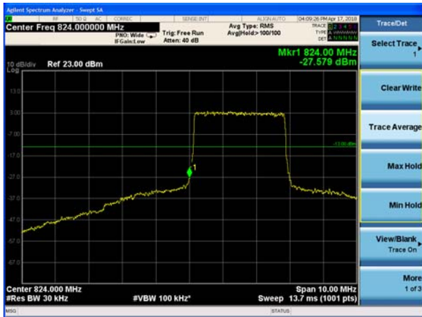
LTE Band 5 16QAM 5MHz CH-Low 1RB
