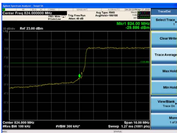
LTE Band 5 QPSK 10MHz CH-Low 100%RB
