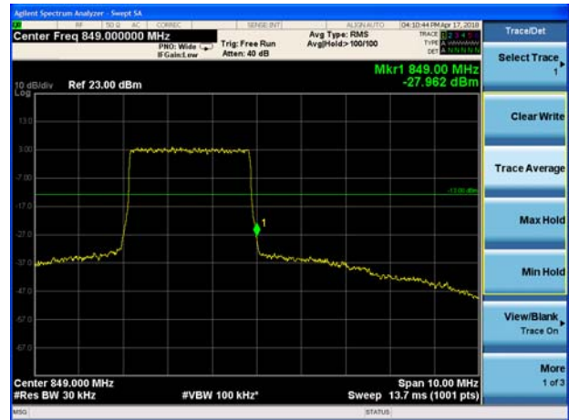
LTE Band 5 16QAM 5MHz CH-High 1RB
