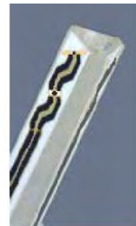
Figure E.2.2 Probe Thick-Film Technique
