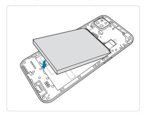
2 Place the battery into the device. Please make sure to place the top portion of the battery before comp letely inserting the battery into the device.
