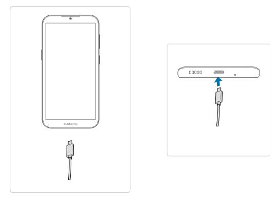
2 Connect the USB cable with power adapter and then plug the charger into a power outlet.
