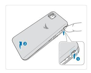
3 Gently press the bottom portion of the batt ery to fully insert the battery into place
