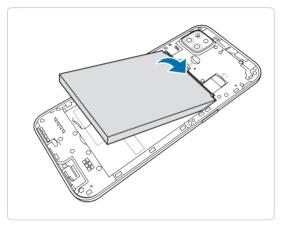
4 Press the battery cover evenly on all sides to connect the battery cover back into place.
