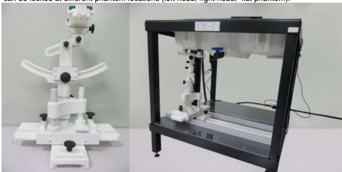
Device holder supplied by SATIMO
