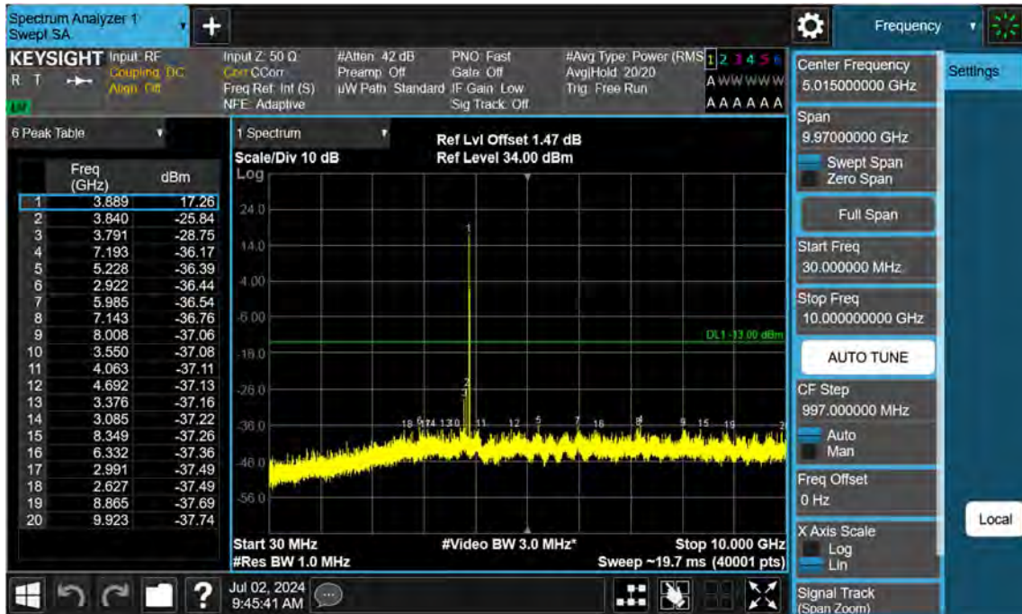
100 MHz / 256QAM / RB Size/Offset (1/Edge Right) – Middle Channel
