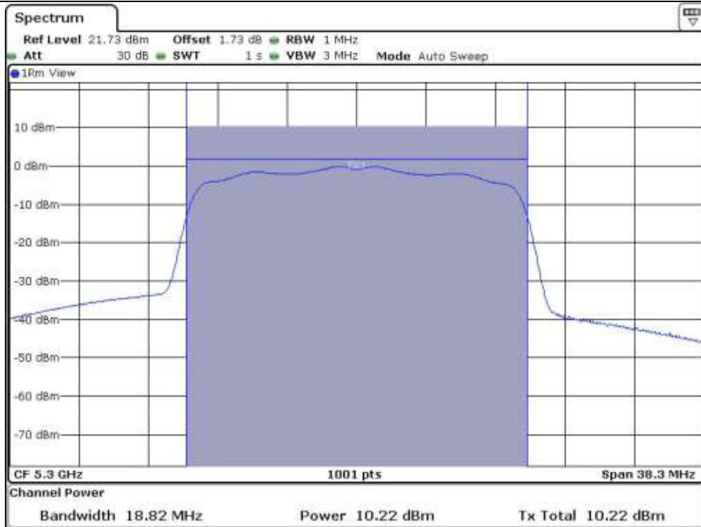
Low Channel @ 5 260 MHz (26 dB Bandwidth)
