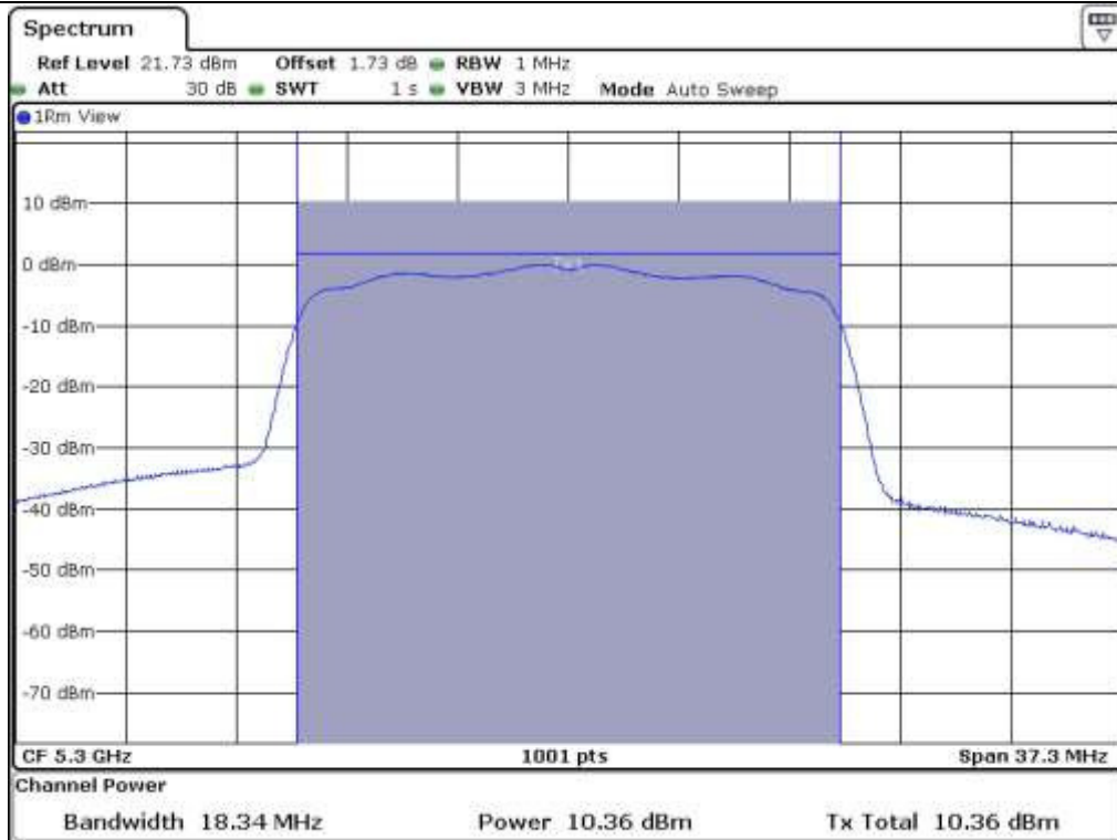
Low Channel @ 5 260 MHz (26 dB Bandwidth)
