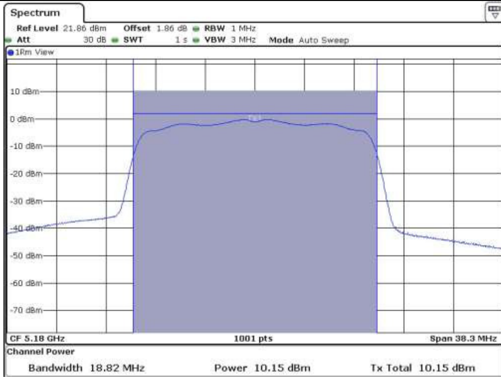
Low Channel @ 5 180 MHz (26 dB Bandwidth)
