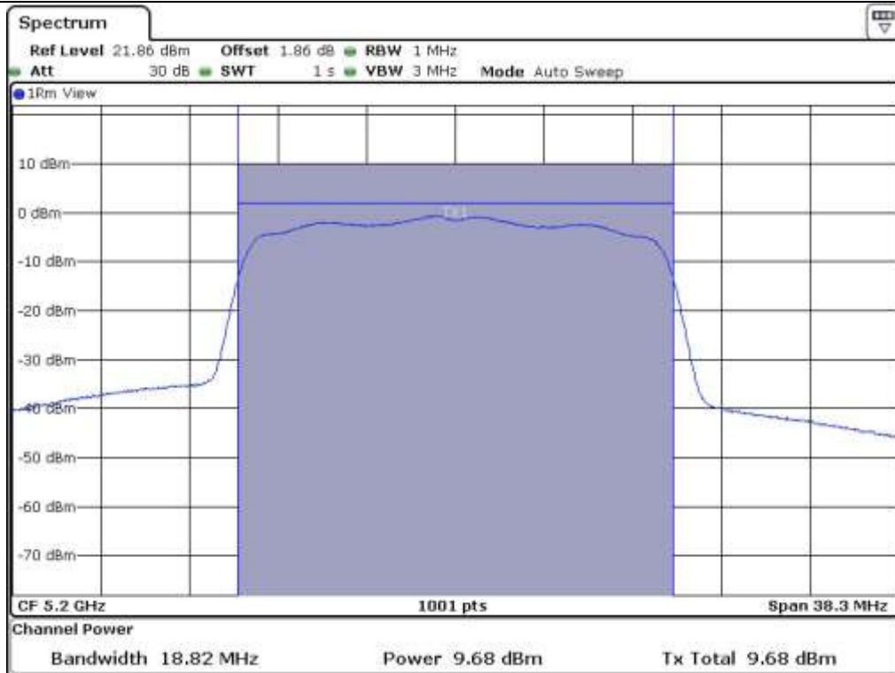
Low Channel @ 5 180 MHz (26 dB Bandwidth)
