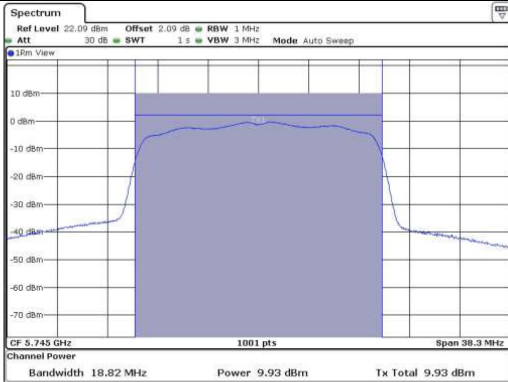
Low Channel @ 5.745 MHz (26 dB Bandwidth)
