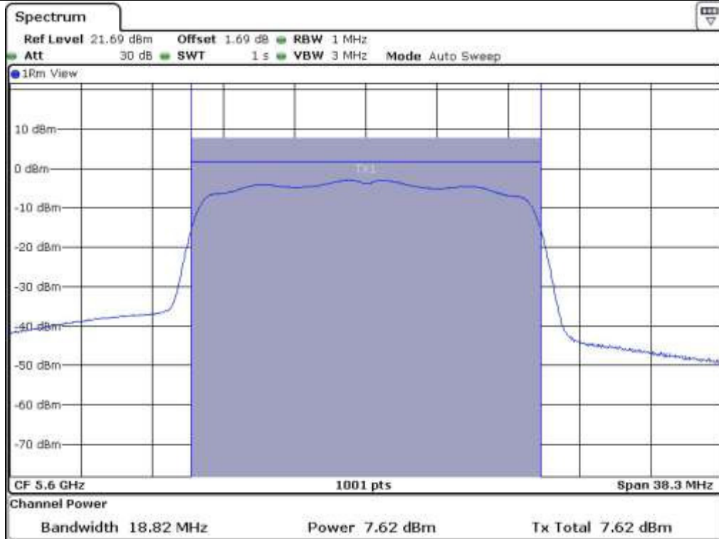
Low Channel @ 5 500 MHz (26 dB Bandwidth)
