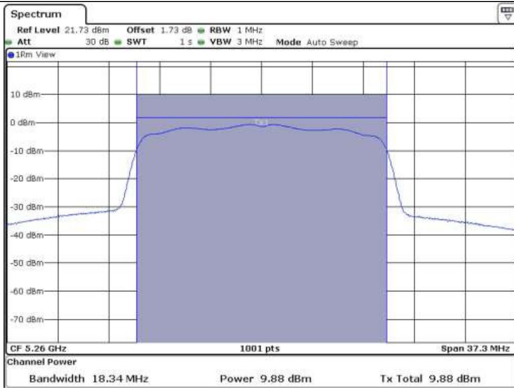
Low Channel @ 5 260 MHz (26 dB Bandwidth)
