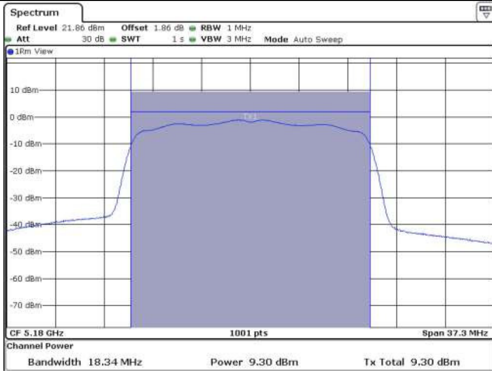
Low Channel @ 5 180 MHz (26 dB Bandwidth)
