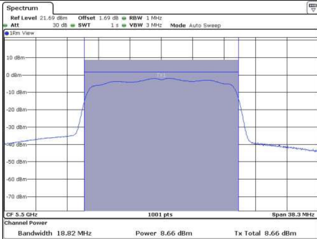
Low Channel @ 5 500 MHz (26 dB Bandwidth)
