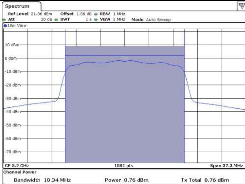
Low Channel @ 5 180 MHz (26 dB Bandwidth)
